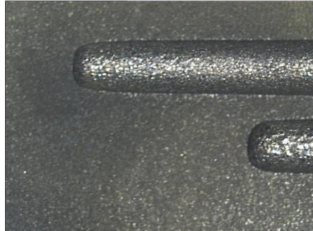
**Fig.4** Spark erosion bores in Ta
