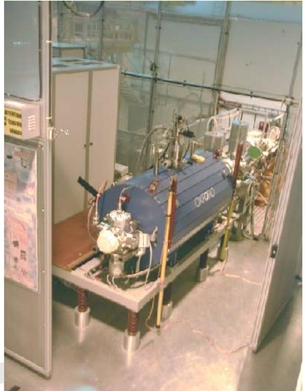
**Figure 9.3 Phoenix ECR ion source (left) and REXEBIS charge breeder (right)**
